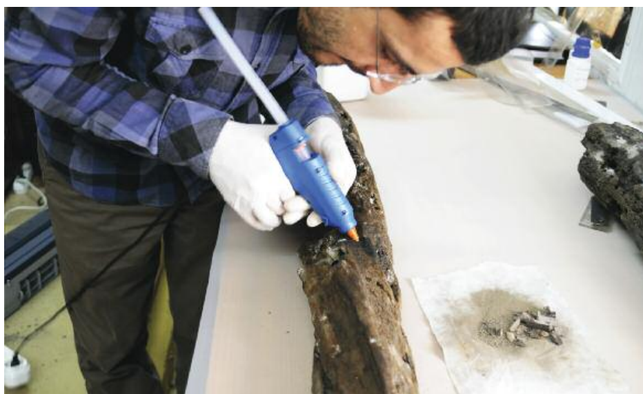
Fig. 4: Bonding procedure for timber components
