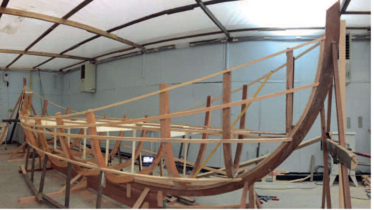
Fig. 22: Gvde biimini belirleyen tirizler. Fig. 22: Battens that designate the shape of the hull.
