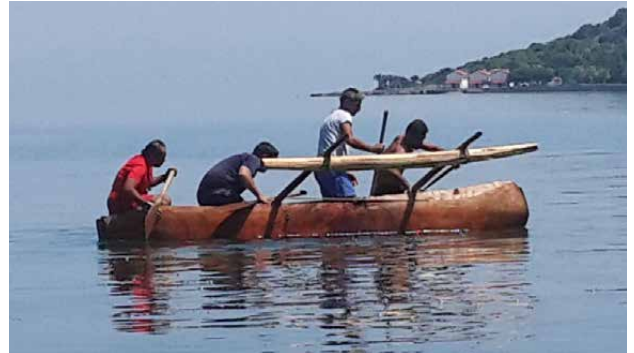
Fig. 14: Tek Denge Kollu Kanonun Performans Denemeleri. Fig.14: Performance testing of the canoe with a single stabilizer.
