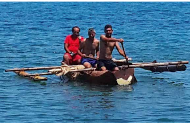
Fig. 15: Çift Denge Kollu Kanonun Performans Denemeleri. Fig.15: Performance testing of the canoe with double stabilizers.
