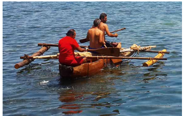
Fig. 16: Çift Denge Kollu Kanonun Performans Denemeleri. Fig.16: Performance testing of the canoe with double stabilizers.
