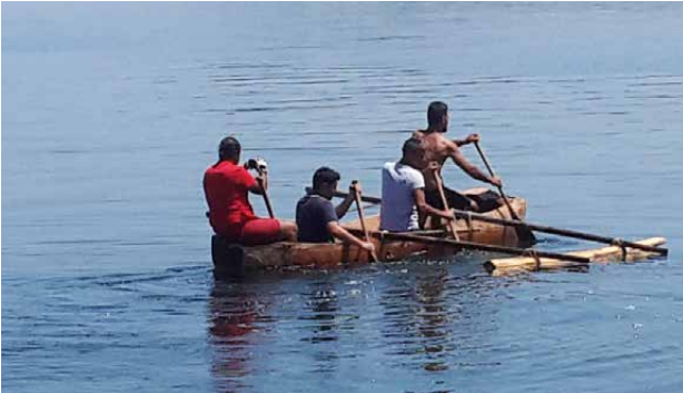
Fig. 13: Tek Denge Kollu Kanonun Performans Denemeleri. Fig.13: Performance testing of the canoe with a single stabilizer.
