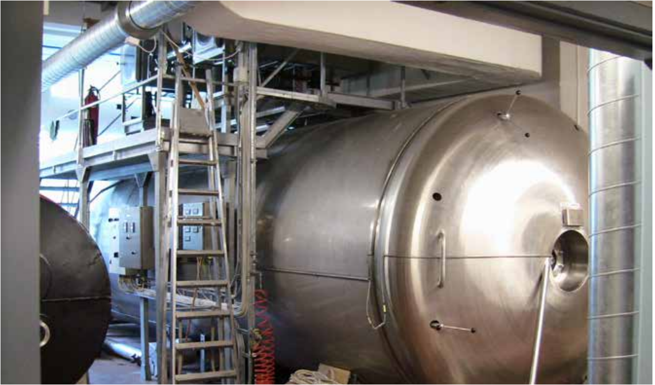
Fig 3: Brede Suya Doymuş Ahşap Konservasyon Laboratuvarı'ndaki vakumlu dondurarak kurutucu, Danimarka/ Kopenhag, 2007 / Vacuum freeze dryer at the Brede Waterlogged Wood Conservation Laboratory, Copenhagen, Denmark, 2007.
