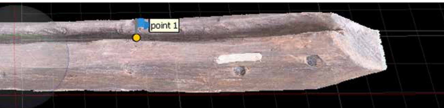
Fig. 5b: Photogrammetry documentation of conserved timbers from the 10th-century vessel YK 24 after conservation using AgiSoft Metashape (M. Jones). The computer program can produce highly accurate three-dimensional models of the timbers before or after conservation, although surface details that may be obscured by the conservation process are more accurately documented beforehand.
